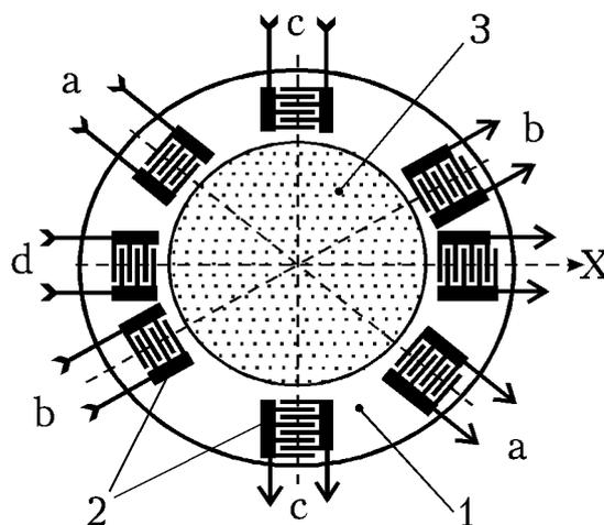
Fig. 1. The integral structure for the investigation of gas phase adsorption upon thin film materials: 1—piezoelectric substrate; 2—interdigital transducers (IDT); 3—a film under investigation; a, b, c, and d—probing channels.
