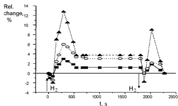
Fig. 2. Temporal changes of density  $\Delta\rho/\rho$  ( $\square$ ) and elastic moduli  $\Delta C_{11}/C_{11}$ ,  $\Delta C_{44}/C_{44}$  of  $Pd_{0.97}Ni_{0.03}$  film during hydrogen adsorption and desorption ( $h = 300$  nm,  $20^\circ C$ ).  $H_2$ —dry air switched off, gas mixture 1%  $H_2 + N_2$  switched on;  $H_2$ —gas mixture 1%  $H_2 + N_2$  switched off, dry air switched on.
